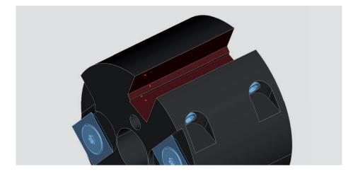
> Clean the base of the cutting inserts [18] using a dry cloth.
