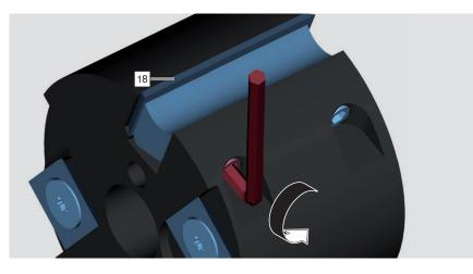
> Loosen the screw for the cutting insert [18] by turning it anticlockwise.
