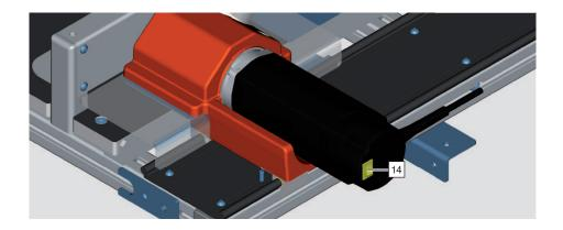
Press the rocker switch [14]. Switch on the motor.
