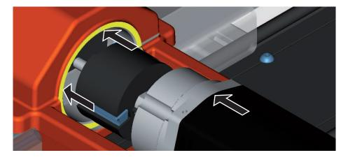
All the fixing and clamping surfaces on the carriage and motor must be free of dust and wood chips.
