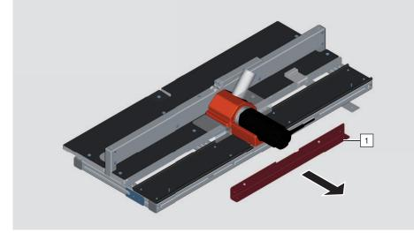
The carriage on the base notching device is secured by the fixing bracket [1].
