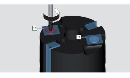
> Loosen the pre-cutter screw [17] by turning it anticlockwise.
