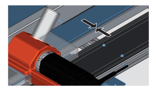
> Push the workpiece against the lateral stop, as shown.
