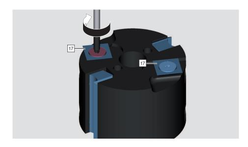
> Tighten the screw in the pre-cutter [17] by turning it clockwise.
