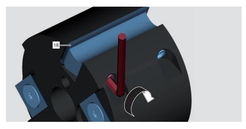
> Tighten the screw for the cutting insert [18] by turning it clockwise.
