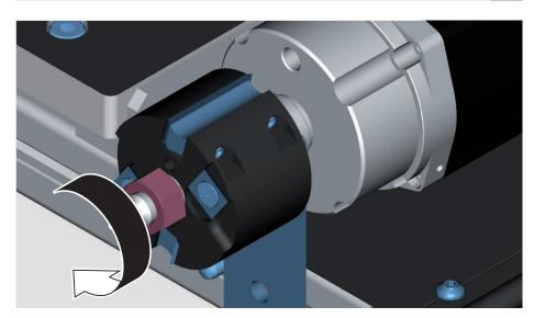
> Turn the nut clockwise using the IM spanner.
