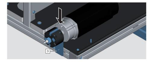
> Secure the motor in the shaft holder [3].
