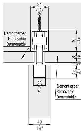
**SoftMove 100 magnetic soft closing mechanism**
