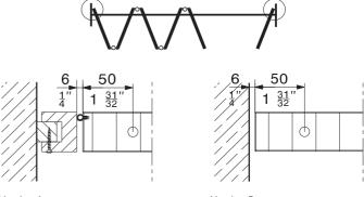
Version A With premises-fitted compensation strip and hollow seal code 19657
