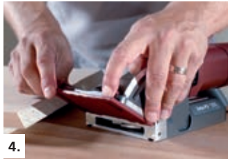
4. Set the swivelling front stop to 60° and attach the 4 mm spacer
