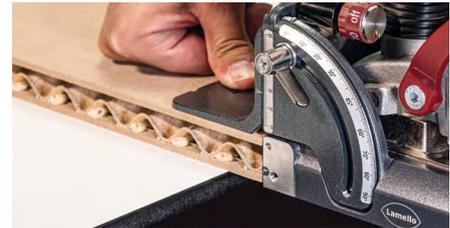
Align the Zeta P2 in the hole using the positioning clip and cut the next groove\*
